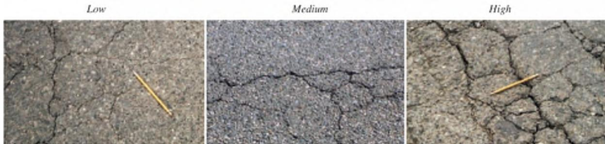
**Figure 8. Alligator Cracking Severities**
